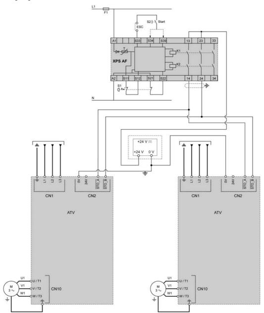
Wiring diagram for frame sizes 4 and 5
