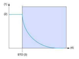
(1) Speed axis - (2) Motor speed - (3)  $\overline{STO}A$  or  $\overline{STOA}$  and  $\overline{STO}B$  or  $\overline{STOB}$  -  $\overline{STOB}$  -  $\overline{STO}A$  ctivation - (4) Time **NOTE:** If delay between  $\overline{STO}A$  or  $\overline{STOA}$  and  $\overline{STO}B$  or  $\overline{STOB}$  is greater than 1 s, the safety function  $\overline{STO}$  is triggered and an error is triggered with the error code **[Safety Function Error]** 5 *H F F*.
