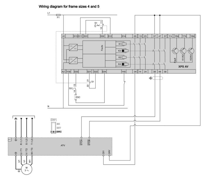
**NOTE:** This diagram is a wiring configuration using DI1 assigned to forward operation.
